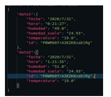
Figure 3. Data model with JSON
