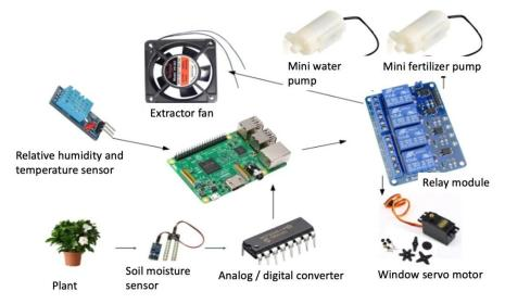
Figure 2. Sensor and actuator connection diagram.
